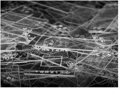
TASTRAK is specifically optimised for nuclear track detection. The plastic is manufactured to high standards and can also be used for optical windows and other specialist applications.
