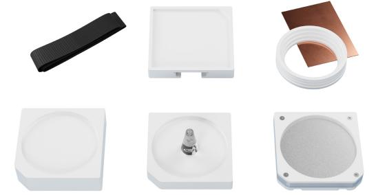
The Pro-Dent set is a universal set of phantoms for carrying out constancy and acceptance tests of conventional and digital dental X-ray units (intra-oral, panoramic and cephalometric).
