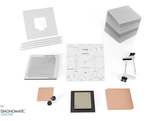
This kit is a versatile set of phantoms and software for carrying out constancy and acceptance tests of radiography x-ray units. Thanks to the Diagnomatic subscription, all tests can be quickly and effortlessly automatically analysed online.
