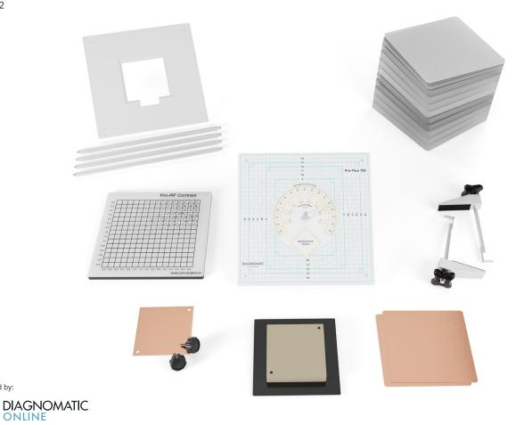
This kit is a versatile set of phantoms and software for carrying out constancy tests of radiography and fluoroscopy units. Thanks to the Diagnomatic subscription, all tests can be quickly and effortlessly automatically analysed online.
